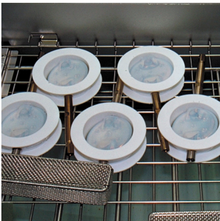
Cleansing the parts with ultrapure water
